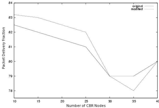
Fig. 5. Impact of Traffic Load: Packet Delivery Fraction vs. Number of CBR Nodes
