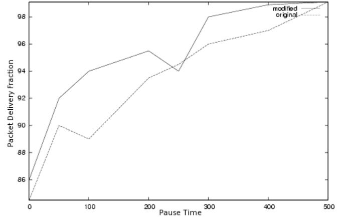
Fig. 3. Impact of Mobility: Packet Delivery Fraction vs. Pause Time
