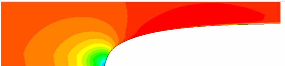
Figure 11(b). Enlarged view of Contours of Velocity Magnitude for DREA Submarine Hull at Re = 23 Million near bow using Unstructured Grid
