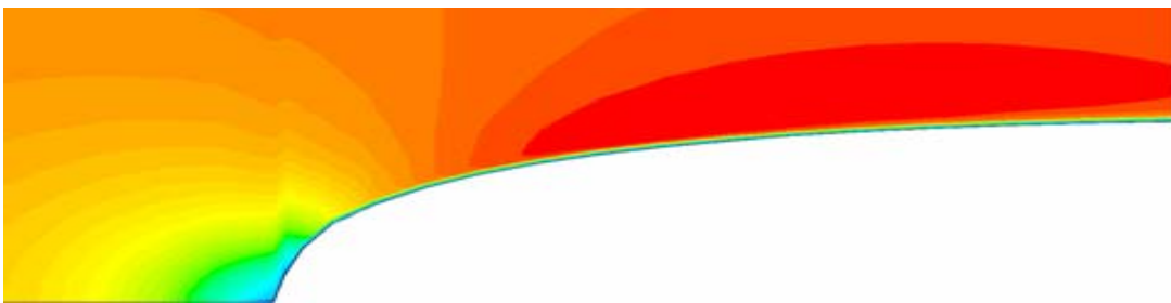
Figure 10(b). Contours of Velocity Magnitude for DREA Submarine Hull at Re = 23 Million using Structured Grid
