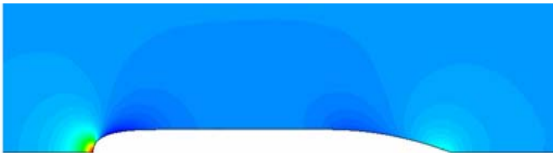
Figure 7(a). Contours of Static Pressure for DREA Submarine Bare Hull at Re = 23 Million using Unstructured Grid
